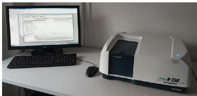
Fig. 14. Absorption spectroscopy setup using the Jasco V-760 UV-Visible/NIR spectrophotometer.
